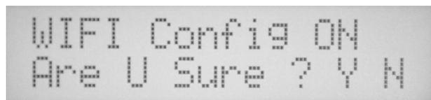
Mode flashing 'W' showing NexPump in WIFI Config Mode.
