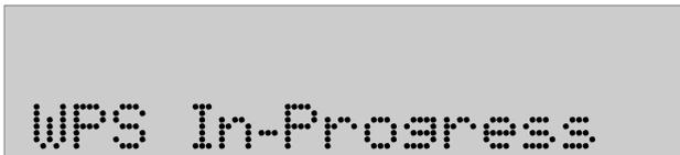
Once the LCD switches to WPS In-Progress, it should take a few minutes to make the connection to your router. Once a connection is made the NexPump will automatically select a Function 'I' for you. The Function 'I' will toggle through many screens. You can verify the wireless connection from the screen SSID Connection: which now should show your SSID. The next screen will show the IP Address of the NexPump, assuming DHCP is enabled.
