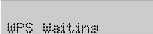
Once the NexPump is in the WPS Waiting Mode, press the WPS Button on the wireless router you would like to have the NexPump connect to. If you are unfamiliar with the WPS Mode of your wireless router, please refer to the routers user manual for more information.
